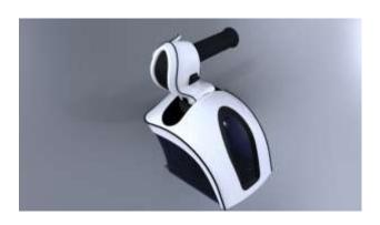
A prototype driving device allows disabled people to steer, accelerate, change gears and brake with one hand (Photo: FICOSA International S.A.)
